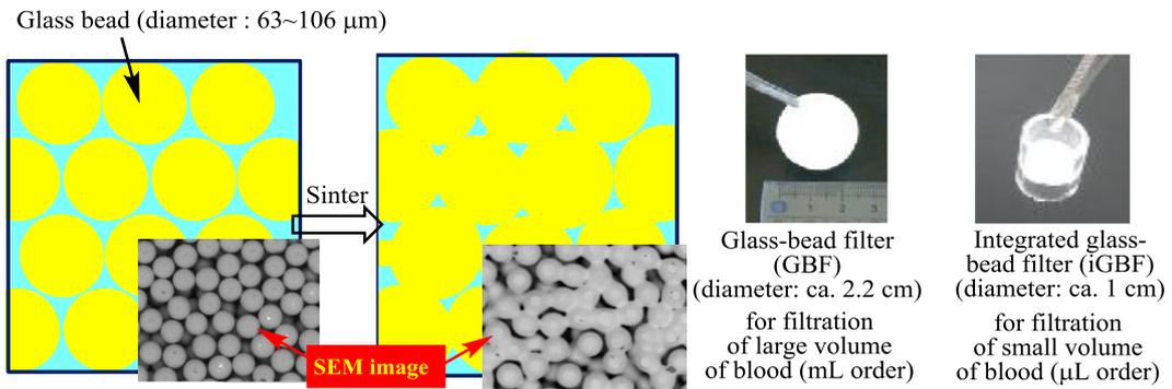
Figure 5. Preparation of glass-bead filter (GBF) by sintering glass beads
